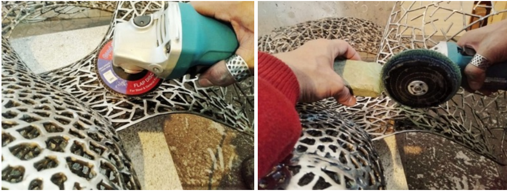
Figure 10. Sanding Using a Stacked Abrasive Flap Disc With 240 Grit (Left). Followed by Polishing Using a Denim Cloth Polishing Wheel, Applied With Polishing Compound (Langsol) and Rubbed Onto the Sanded Stainless Steel Surface (Right).
