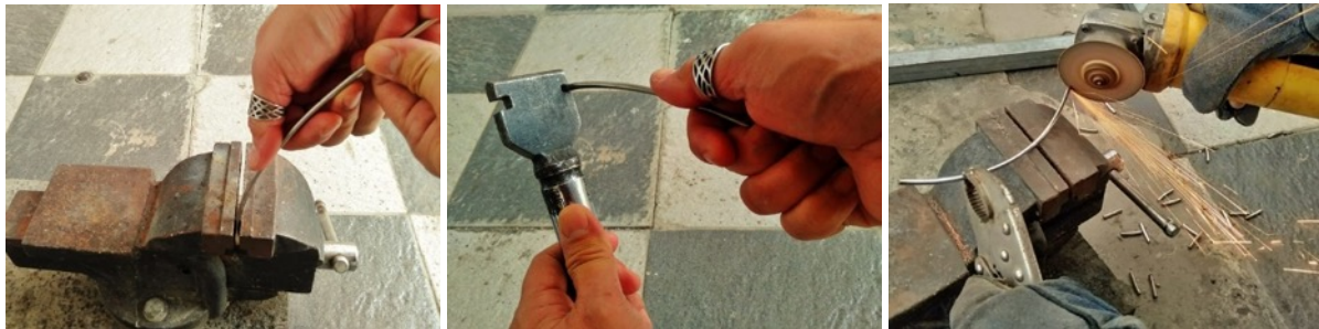
Figure 4. The Process of Bending Stainless Steel Rods Using a Vise (Left). The Process of Bending Stainless Steel Rods Using a Metal Bending Tool (Center). The Process of Cutting Stainless Steel Rods Using Locking Pliers and an Angle Grinder (Right). [Source: Research Team, 2025]
