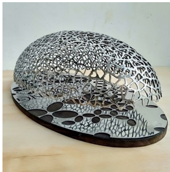
Figure 1. The Result of Welding Stainless Steel Rods into Organic Oval-Formed Curves. [Source: [9]]
