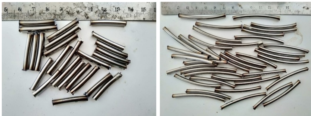
Figure 5. Stainless Steel Rod Segments With a Length of Approximately 2.5-3 cm (Left). Stainless Steel Rod Segments With a Length of Approximately 4.5-5 cm (Right). [Source: Research Team, 2025]
