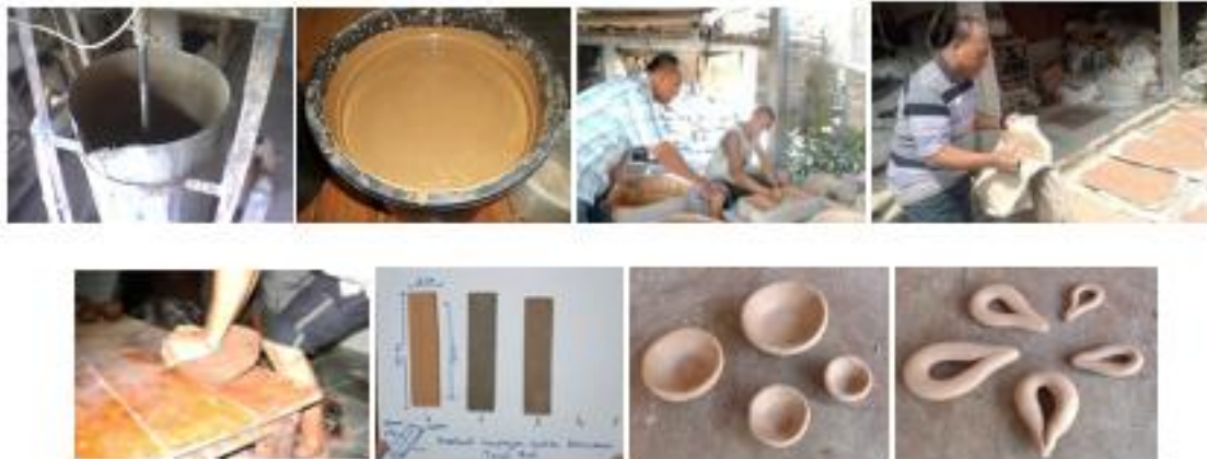
Figure 6. Testing Kasongan Clay in Technical Ceramics to Increase the Strength of Burning Temperature Impact on Ceramic Body Strength [Source: Arif Suharson, 2024]
