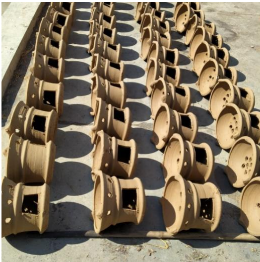
Figure 2. Anglo . The top part holds the load with horizontal protrusions at the four corners to place the load (cooking utensils), and underneath there is a container for charcoal as fuel for cooking. There is a hole to dispose of the remaining charcoal burning on the bottom part. Anglo is often found in wedangan (street food stalls) in Solo and the surrounding area (Source: Personal Documentation, 2021.)
