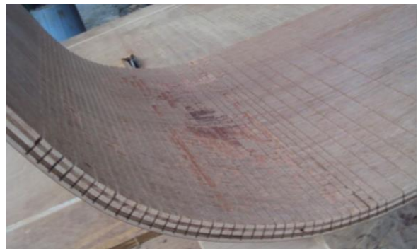
Figure 3. The process of making a drum body from plywood
