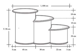
Figure 4. The basic shape of the corner table design (Source: Author, 2016)
